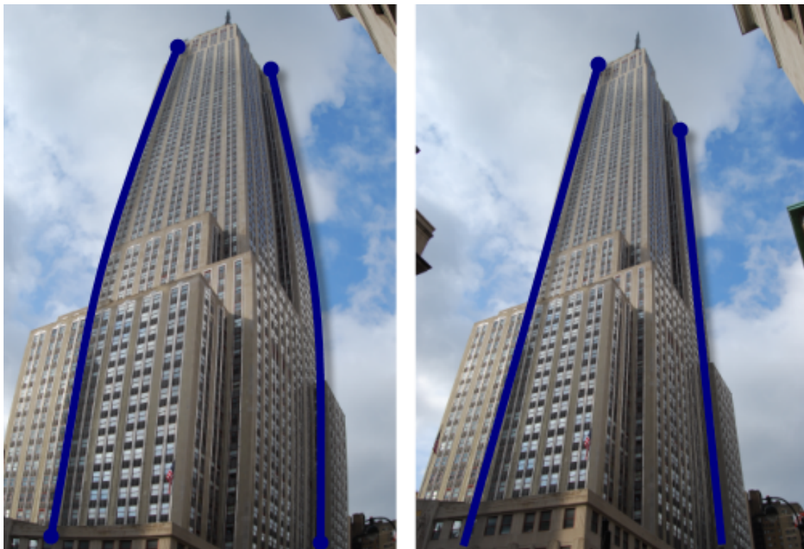
Figure 17: Barrel Distortion or Fisheye Effect (permission pending from MathWorks)
